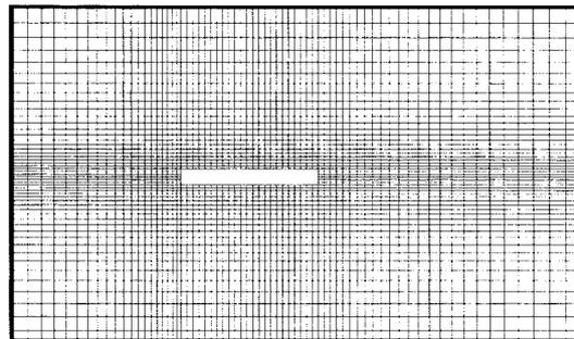
Fig. 2 Finite element mesh in the vicinity of the rectangular section
