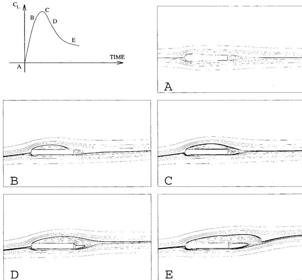
Fig. 8 Time development of the aerodynamic flowfield around the rectangular section
