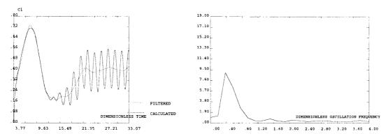
Fig. 6 Indicial lift response and Admittance function, rectangular section
