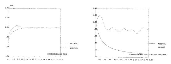
Fig. 7 Normalized indicial lift response and Admittance function, bridge deck section
