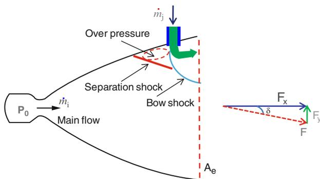
**Fig. 1** Schematic view of fluidic thrust vectoring
