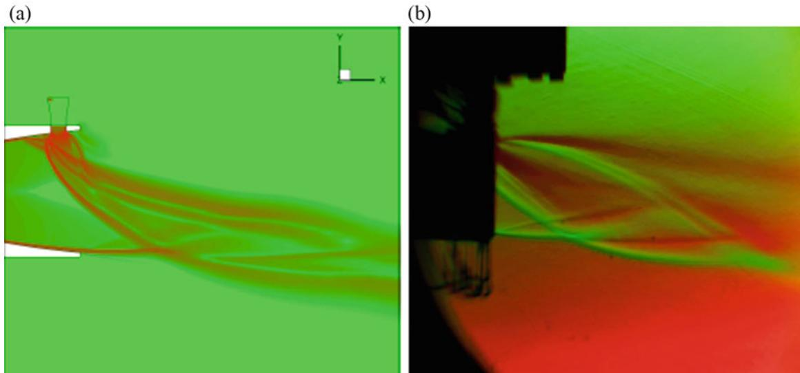
**Fig. 4** Numerical (a) and experimental (b) Schlieren for SPR = 1 (CO<sub>2</sub> into Air)
