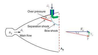
Fig. 1 Schematic view of fluidic thrust vectoring
