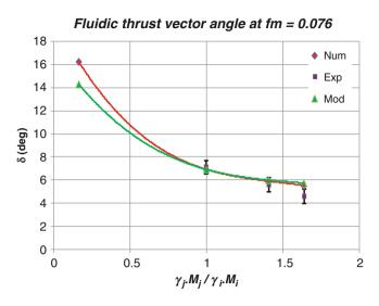
Fig. 6 Fluidic thrust vectoring angles
