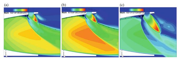
Fig. 5 Mach contours plots, (a) Ar-Air, (b) CO<sub>2</sub>-Air, (c) He-Air, in symmetry plane of the TIC nozzle at  $f_m = 0.076$
