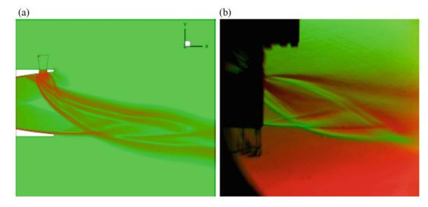
Fig. 4 Numerical (a) and experimental (b) Schlieren for SPR = 1 (CO<sub>2</sub> into Air)
