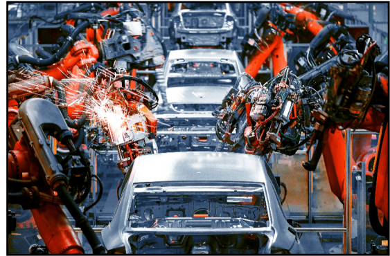
Fig. 1. Automotive BiW with several robots sharing the same workspace.
