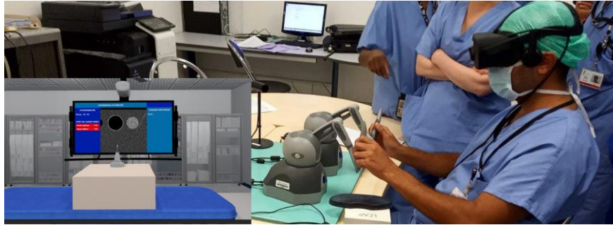
Figure 1: The user interface of the immersive ultrasound-guided locoregional anesthesia simulator. (Bottom left) The Virtual scene with the virtual instruments manipulated by the user and the ultrasound screen displays the ultrasound image.
