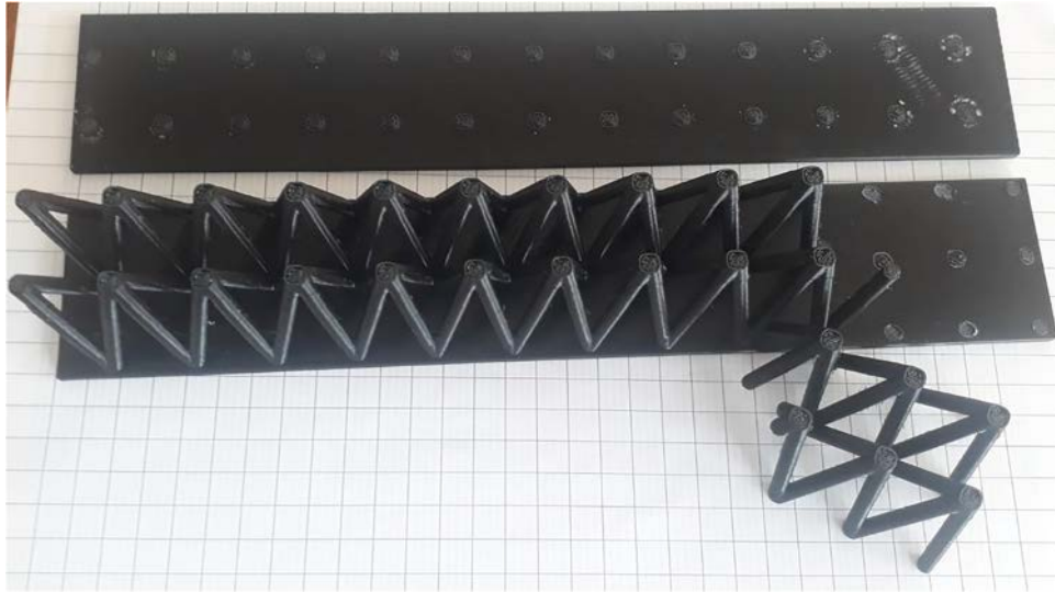
Figure 8. Rupture aspect for the pyramid core sandwich panel.
