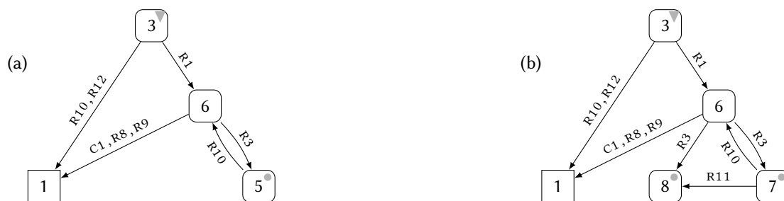
Figure 4: (a) A topological decomposition of the state-space of the termite model where component 3 is the set of initial states (hence its ▼ decoration), component 1 is the set of deadlocks (hence its square-shape), component 5 is the sccs hull (thus it has at least a scc, hence its • decoration), and component 6 is the basin to components 1 and 5. (b) Decomposition of component 5 from (a) into components 7 and 8 with respect to either one-way rule R11, or CTL formula \varphi_{\text{may-die}} \stackrel{\text{df}}{=} \text{EF} \neg(\text{Rp} \vee \text{Wk} \vee \text{Sd}) .
