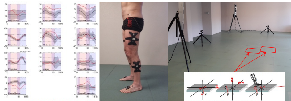
Figure 2. CMA of lower limbs. Different types of sensors are used to conduct kinematic and kinetic analyses of locomotion in gait labs. These include accelerometers, gyroscopic sensors, magnetometers, force platforms, MoCap systems.
