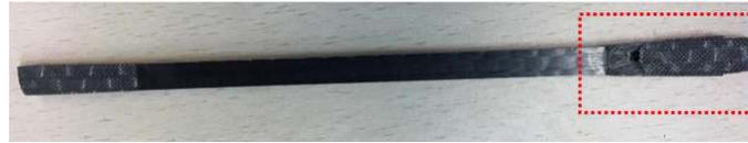
FIGURE 9 – Éprouvette orientée à 0° de  $[C_{10}]$  à rupture
