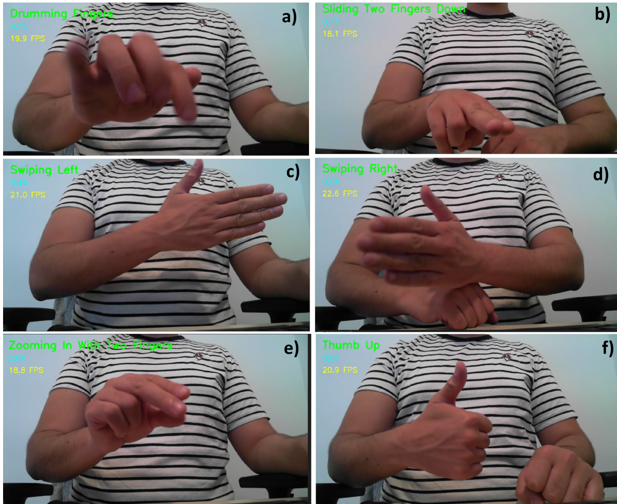
Figure 7: Qualitative hand-gesture inference examples in our RGB-only MR prototype. Predicted class and per-frame confidence (top-1 softmax) are overlaid in cyan. Gestures: (a) Drumming Fingers, (b) Sliding Two Fingers Down, (c) Swiping Left, (d) Swiping Right, (e) Zooming In With Two Fingers, (f) Thumb Up. Yellow text shows the end-to-end camera loop rate on our prototype laptop; this is not XR-SoC throughput.
